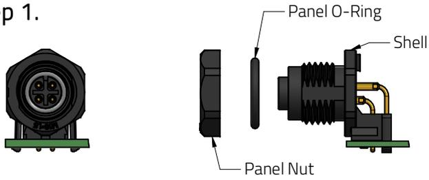
**Step 2.** Install Shell with Panel O-Ring on panel.
