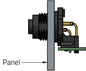
**Step 3.** Recommended tightening torque : 10-15 kgf-cm
